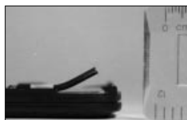
Figure 2: Triggered NiTi actuator displacement for product separation
